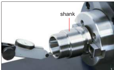
measure radial runout of shank
