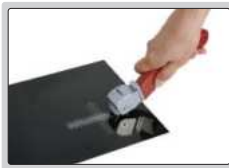
step 1: make grid cutting on surface
