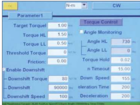
interface of tightening parameter setting
