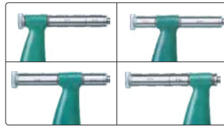
adjust collars for different measuring ranges
