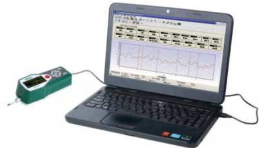
operate roughness tester by computers
