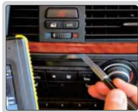
measuring gaps on the car dashboard
