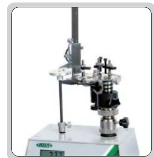
check the measuring force of calipers
