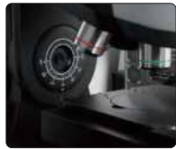
side camera shows the relationship between the lens and the workpiece, reducing the risk of collision
