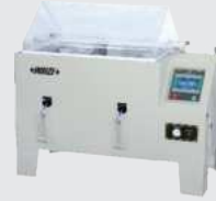
SALT SPRAY TEST CHAMBERS
