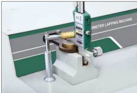
lapping measuring surfaces of caliper lower jaws
