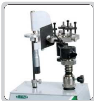
check the measuring force of indicating micrometers
