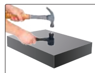
hammer impact to apply test force
